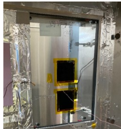
Figure 2. U-value field testing method validation using NLR IGU test chamber.
